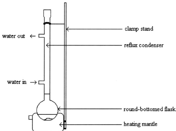
Fig. 11 Esterification apparatus
