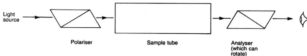
*Figure 1.4 A schematic representation of a polarimeter<sup>15</sup>.*
