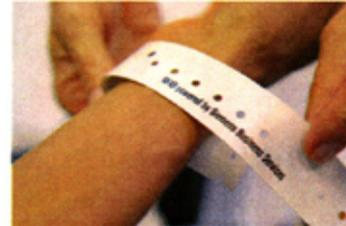
**Figure 3:** An RFID tag is embedded in the traditional patient wristband.
