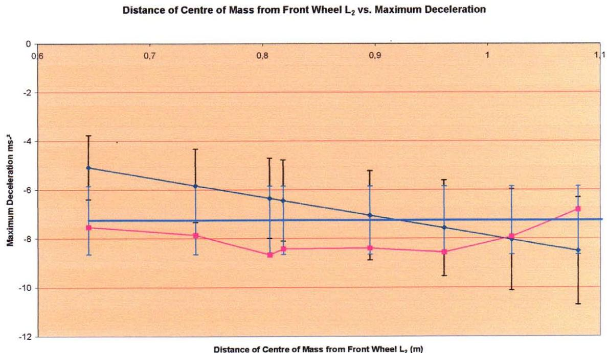
1. One data point differs from the others by lying above the blue line. This is because this limit is for all the weight of the bike being used as the normal force, but for this reading the bike didn't even begin to tip, thus a great deal of weight was about the rear wheel and the normal force was not being exploited for decelerating – this made the bike skid at a lower deceleration.
