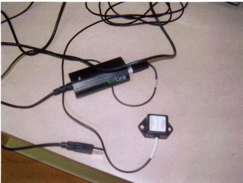
The hardware used to measure the accelerations when braking on the bicycle. The small sensor would be mounted on the handlebar, whilst the rest would be in the backpack.
